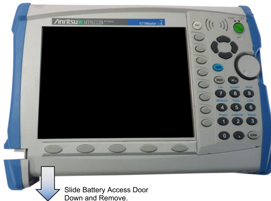
Figure 6-3. Removing the Battery Access Door
